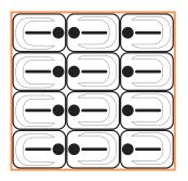
If you prepare liquid packagings in stacks on a skid, place heaviest units at the bottom and stack gradually up to the lightest. Separate layers with wooden planks or thick fiberboard/plywood sheets. Consider overall stability and strength against crushing. Consider banding around each layer.
